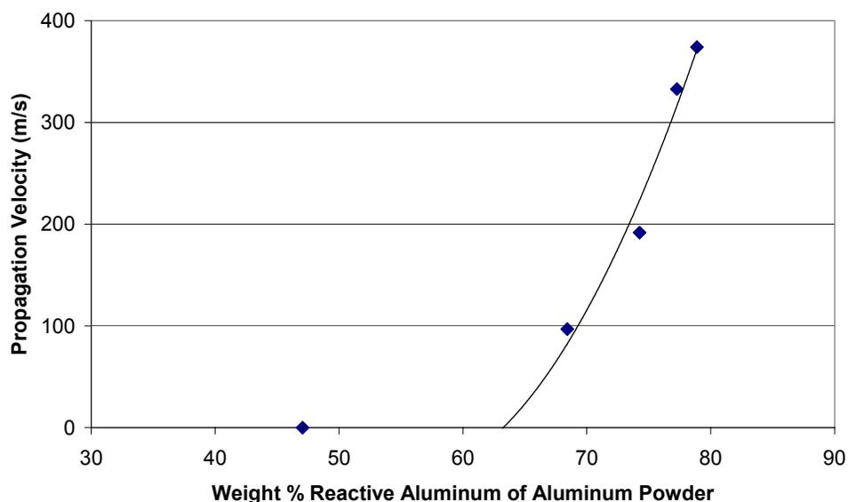
Figure 1: Propagation velocity vs. reactive aluminum content in Al/CuO system. Aluminum nanopowder aged in 97% RH in air.
