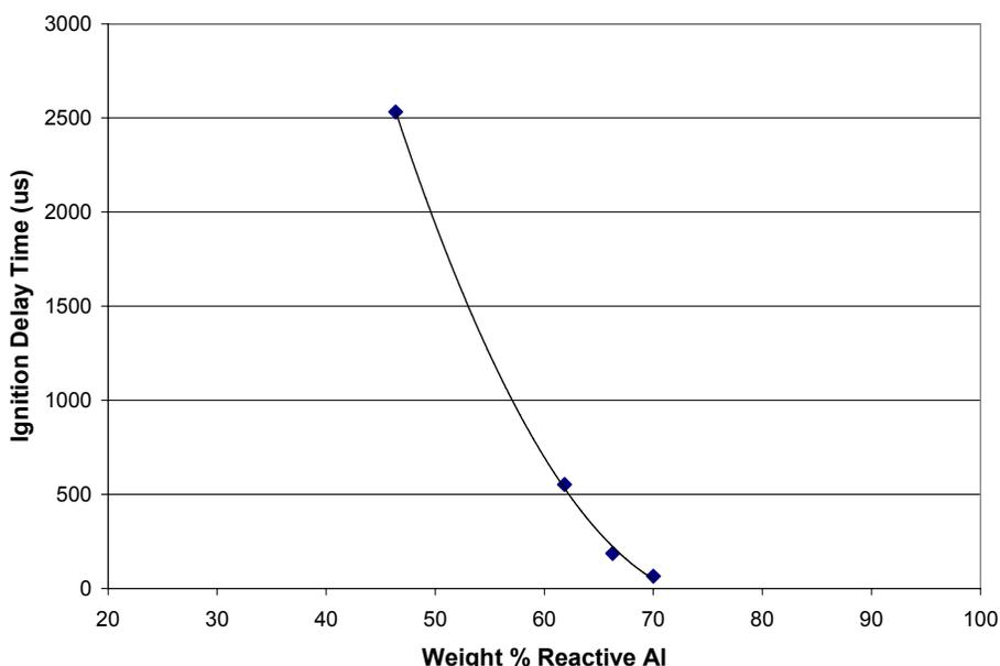
Figure 3: Ignition delay times as a function of weight % reactive aluminum in the Al/CuO system.
