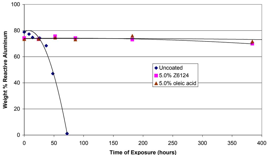
Figure 2: Aging of 80 nm Nanotechnologies aluminum with 5 wt% coatings of Z6124 silane and oleic acid. Aging results for an uncoated sample are provided for comparison. Aging was done in 97% RH in air.
