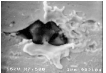
Fig. 19 EV strike on a deuterium loaded palladium foil.
