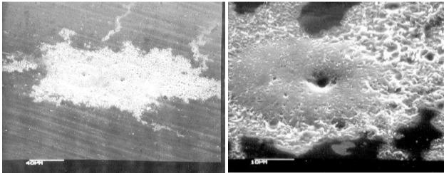
Fig. 8 Aluminum oxide deposited on 6 micrometer thick aluminum from EV boring through aluminum oxide.
