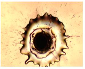
Fig. 5 Optical micrograph of EV entrance into lead glass showing wave action of sloshing.
