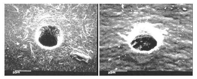
Fig. 12 Entry side of an EV strike on silicon carbide grain coated on a 0.001" thick aluminum foil.
